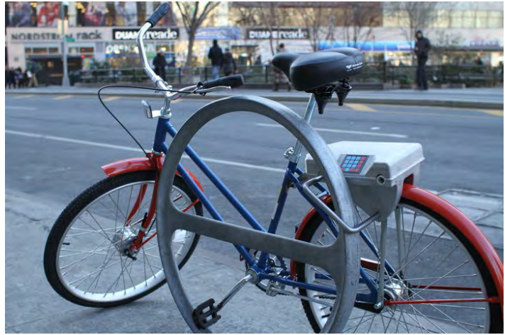
Image of a station-less bike share bicycle, with independent locking mechanism (Source: The Social Bicycle Company)
